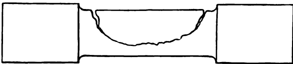
Fig. 11—Characteristic break of a hardened steel test piece
